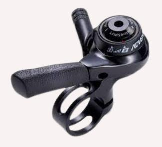
Most common one and easiest to use, as the person cycling can still hold the bar well, while pushing the levers only with the thumb. There are hundreds of models and series, so if replacing one it is important to check compatibility.
