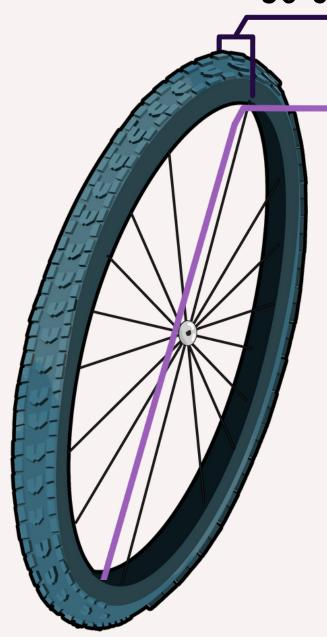
559MM (FOR 26 INCH TIRE) 584MM (FOR 27.5 INCH TIRE) 622MM (FOR 29 INCH TIRE)
